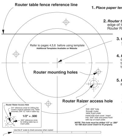
**6" Scale.** If template is copied or downloaded from web site, use this scale to accurately check template size.
